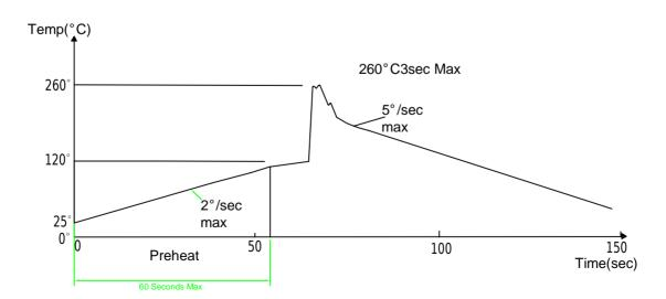
Note: 1. Wave solder should not be made more than one time.
